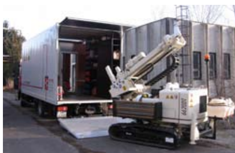
(right and above) Although their 6620DT is only a few months old, the geo-log machine has traveled extensively, secure in the MAN transport truck. The 6620DT started a project in eastern Hungary during the winter. The machine is loaded into the truck via a hydraulic ramp. The MIP equipment is situated in a "clean room" in the front of the truck.
