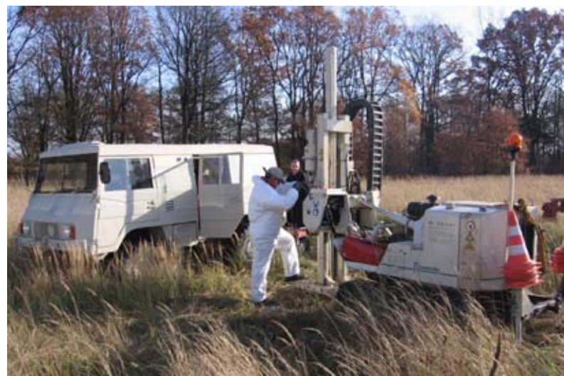
A 6610DT pushes cabled MIP rods (housed in the Pinzgauer Type 710K) at an abandoned airfield in eastern Germany. The Pinz is the dedicated MIP vehicle for geo-log.
