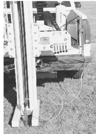
Post-Run Tubing (PRT) connected for soil gas sampling.
